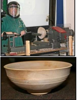
He formed a break between the curve of the bowl and the start of the curve of the rim using a 3-point tool. Then, with a 3mm beading tool he cut 3 beads; the tool is used by starting with the handle low, then slowly raising it as the cut progresses. He used a 3M abrasive bristle disc in a drill to clean up the beads. The external shape can be seen in the photo.
